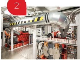
Diesel generators and electric motors are a successful combination for the Farge, a vehicle and passenger ferry that crosses the Weser river in Germany
